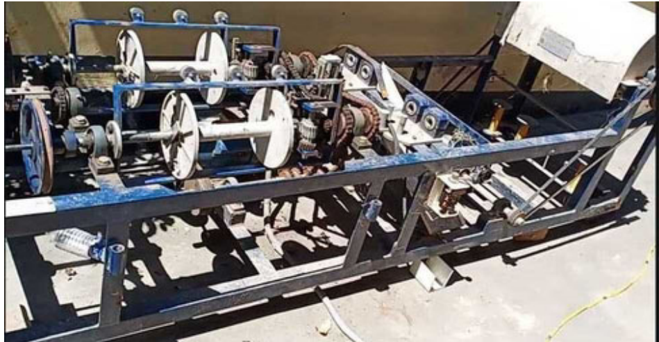
Fig.4: Coir Jute fiber shredder machine
